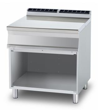
Construction - Fabricated using CrNi 18/10 AISI 304 grade Stainless Steel Scotch-Brite Satin polish Finish, incorporating 2mm thick worktop, rounded edges, chromed details and rear splash back. Model -Professional worktop with or without drawer on open cabinet. Fittings -Appliance is supplied with steel or plastic tanks, h 15cm. Adjustable feet. Doors not included.
